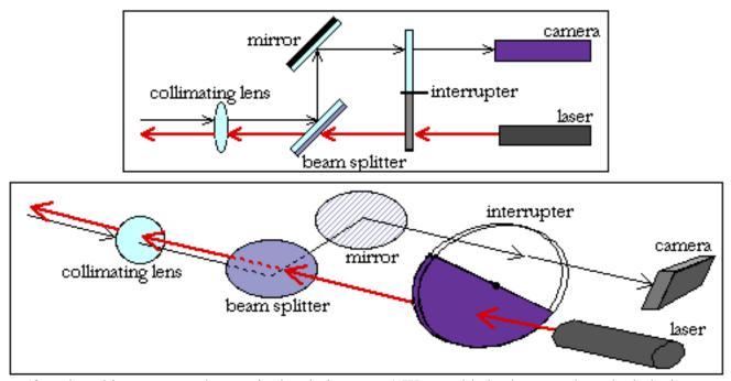
50%, then this argument changes in the obvious way.) We would also have to phase-lock the interrupter to the imager; this might require a phase-locked-loop and a position encoder (trivial to do, given this spinning light-and-dark disk), or possibly some sort of brushless DC motor driver.
