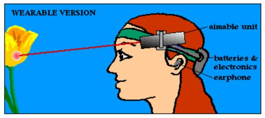
This approach is more convenient than a completely manual tracking system, since it frees both hands and enables two-eyed viewing. It still requires the user to carefully position a laser spot on the target, hence essentially fixing the orientation of the eyes relative to the head when the user wishes to scan something. While somewhat inconvenient, this is still much easier than a manual tracker, and still relatively easy to build.
