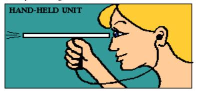
The imager (see details in the description of the primary imaging system in section A.1) can be simply positioned in a fixed relationship inside the collimating tube shown, making the design easy. Unfortunately, this requires one-eyed use (most people close one eye when sighting through something), and also ties up a hand. This is the least desirable configuration from the viewpoint of ease-ofuse.
