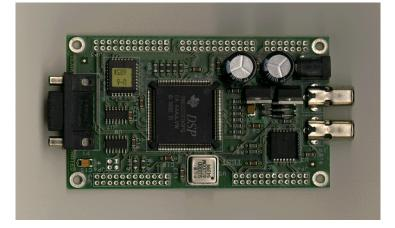
75% of actual size; the actual 6 by 10 cm unit is one-half of what gets head-mounted (the other half, of course, being the optical system, on the other side of the head for balance).
