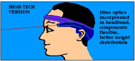
The use of optical fiber would tend to automatically collimate the incoming light, though it is also important to use a suitable lens to gather enough light, and to match it to the narrow diameter (typically 100 microns or less) of the fiber. Similarly, a fiber optimized for visible-light operation is necessary; most are optimized for the near-infrared.
