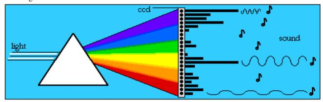
run it through a prism to spread its spectrum, and then run the resulting fan of light into a one-dimensional CCD imager.
