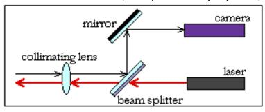
Note well that, in the diagram above and in most of the diagrams here, the box labelled *camera* is actually a combination of a prism or grating of some sort and a camera.
