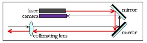
This diagram is simplified; for example, it doesn't include the beamsplitter, associated mirror, and possible interrupter (all of which would be in the upper optical path), and the pair of mirrors at the right would more likely be a single right-angle prism. This setup could put the bulk of the components parallel to the collimation path, hence shortening the whole thing.
