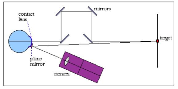
The original purpose of such an apparatus is to stabilize an image on the retina no matter how the eye moves; such a stabilized image almost immediately fades out. By turning the former projector into the imaging system instead, we can always see what the user is seeing, no matter how his eye moves—with some important provisos.
